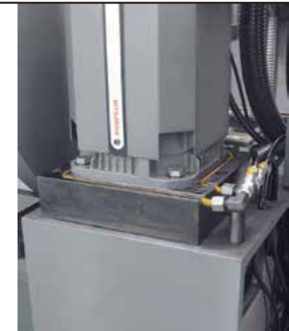
Direct Type Spindle Motor Cooling Device
